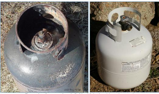
Example of a rusted tank (left) which should not be used, and a fully serviceable tank (right) which should be
